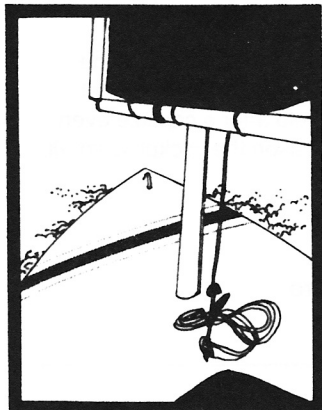
This picture shows halyard cleated, coiled, and properly secured for sailing.
